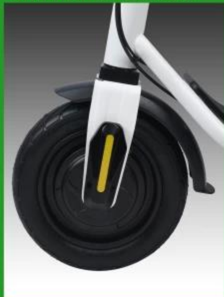
Front wheel E-ABS 8.5-inch Tubeless tire
