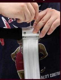
Put the clamp cover back, and fasten it with screws.
