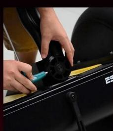
Insert handlebar into the padel base, then fasten the hexagon screws.
