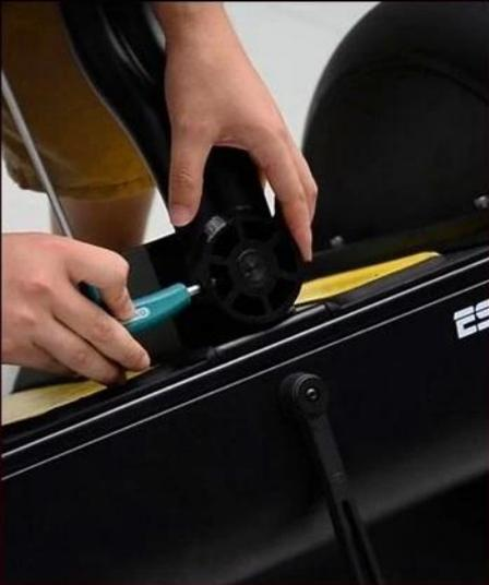
Insert handlebar into the pedal base, then fasten the hexagon screws.
