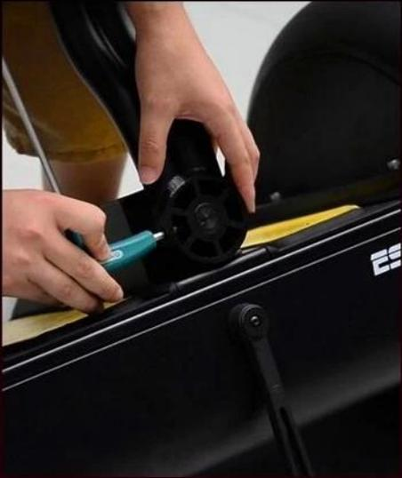
Insert handlebar into the pedal base, then fasten the hexagon screws.
