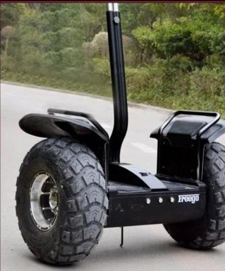
Keep the scooter remain level, then switch the power on.
